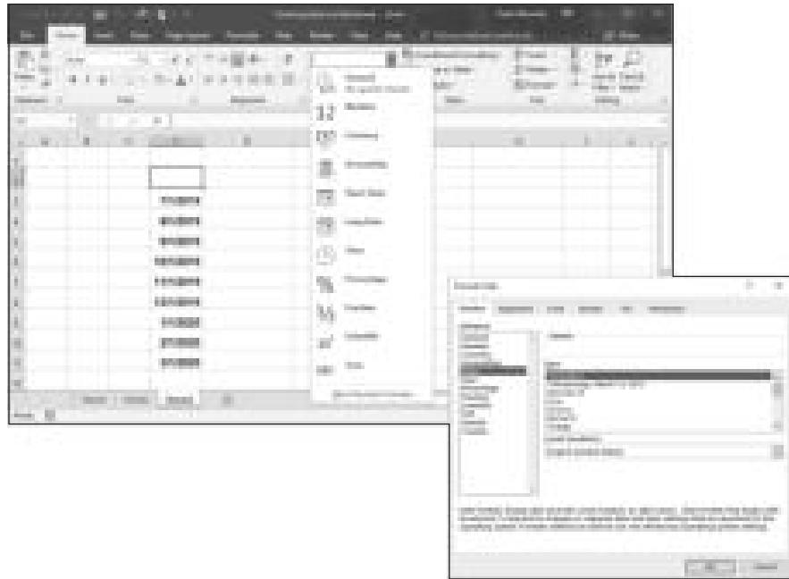
FIGURE 1-5: Format dates and numbers on the Number Format drop-down list or Format Cells dialog box.
